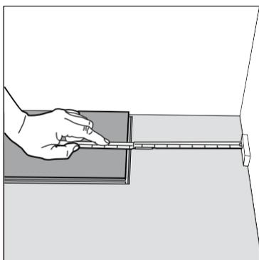
③ At the end of the first row, leave an expansion gap of 1/4" to the wall and measure the length of the last plank to fit.
