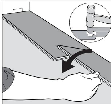
② Second Plank, first row. Drop the plank and gently press down the end with a rubber mallet so it firmly locks into the previous plank until both are at the same height. Make sure both planks are perfectly aligned. NOTE: If you notice both planks aren't at the same height or are not well locked together, please follow the disassembling instructions at the bottom of the page, disassemble and check if any debris stuck inside the lock is obstructing.
