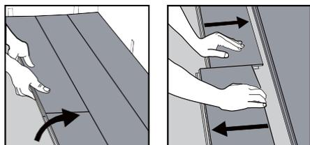
Separate the whole row by lifting it up delicately at an angle. To separate the plank end-joints, leave them flat on the ground and slide them apart. If planks do not separate easily, you can slightly lift up the planks (5° angle) when sliding them apart.
