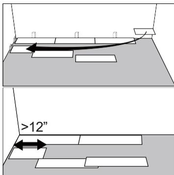
⑤ Start the second row with the leftover cut part of the last plank of the previous row. This small plank should measure at least 12". Otherwise, use another plank that should be cut in two. The end joints of each adjoining row should not be closer than 8" to each other.
